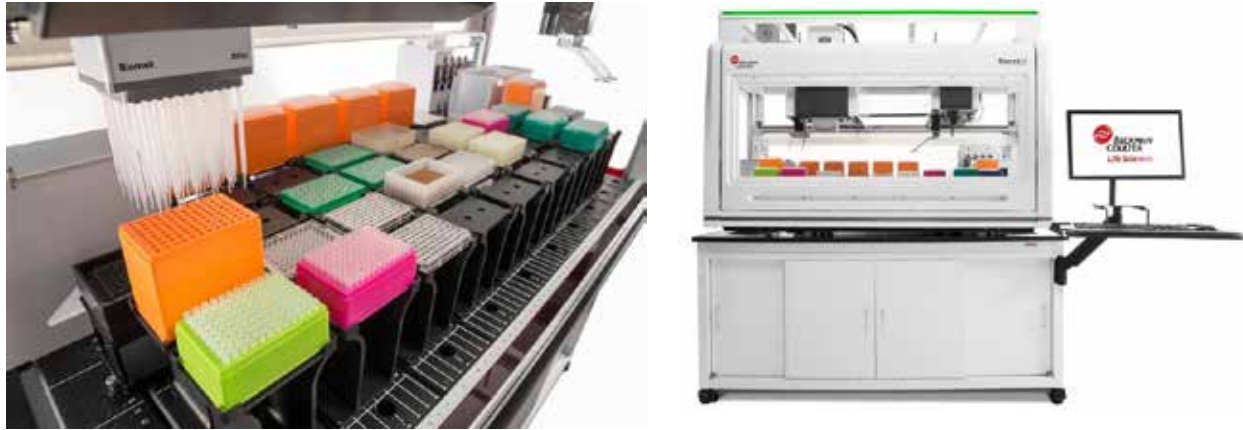
Figure 1. A picture of a representative deck layout of a Biomek i7 Hybrid Workstation and a photo of the workstation.
